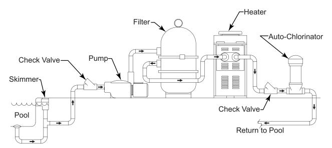
Figure 1. Pool/Chlorinator Setup.
